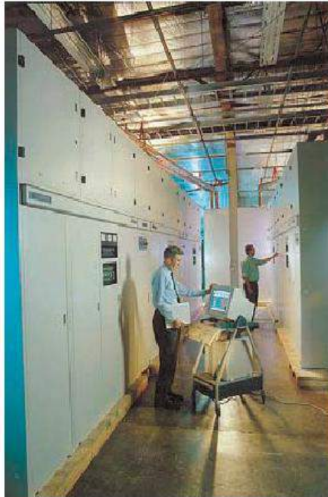
Hilmer Swanson checking the operation of a DX-1000 (TPO: one million Watts)
